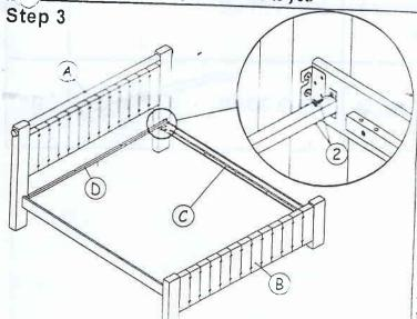
ix cross bar 'D' to the side rail with bolts '2' as shown.
