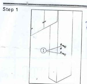
Fix screw '1' into position on wood post as shown. Important note: Do not tighten the screws yet!
