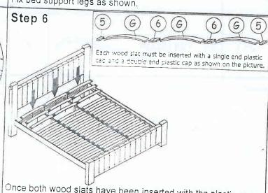
Once both wood slats have been inserted with the plastic caps, fix it on the wood side rails and center bar by pressing it accordingly to the default holes. Ensure the plastic caps pin is aimed to the holes.
